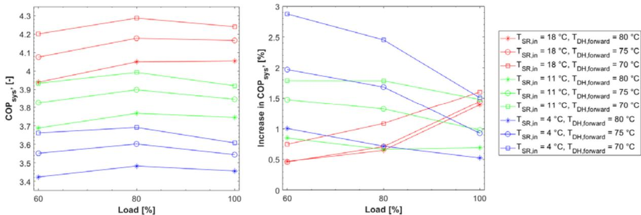
Figure 7: Left: System COP based on optimized set points. Right: Improvement compared to initial settings
