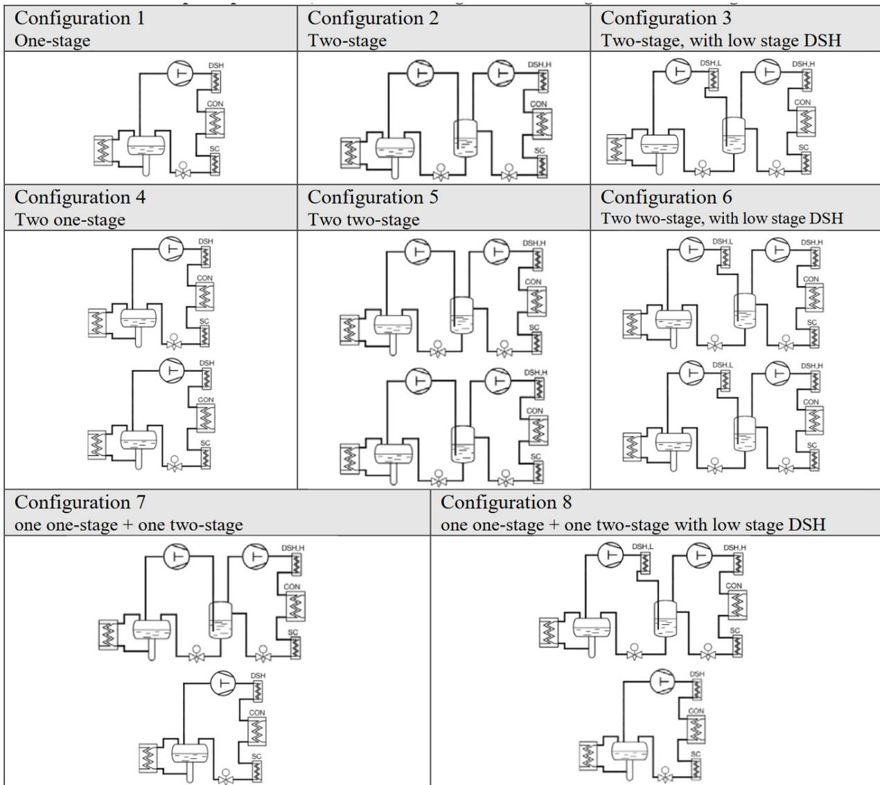
Figure 8: Compared configurations
