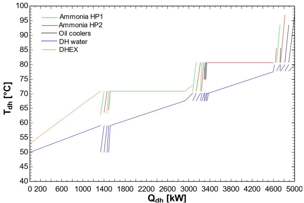
Figure 11: Optimized two-stage configuration for geothermal source ammonia heat pump
