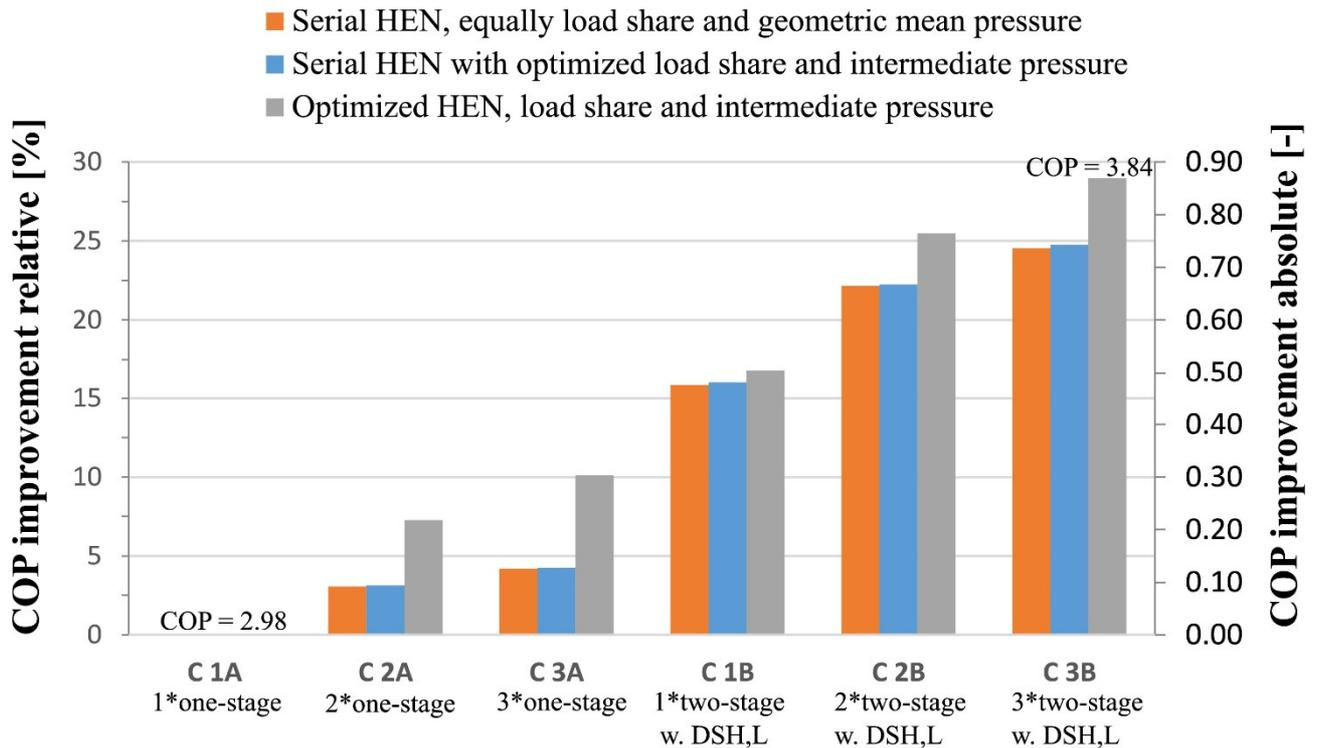
Figure 4: Comparison of configurations and COP optimization potential.
