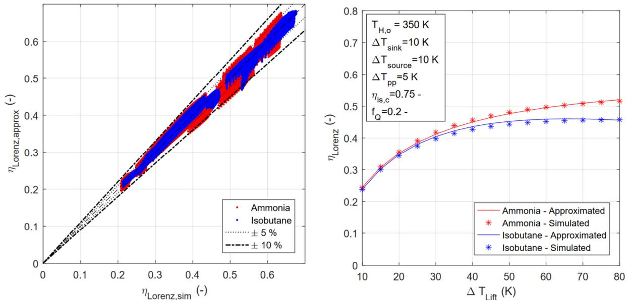
Figure 6: Comparison of estimation and detailed simulation value of heat pump COP
