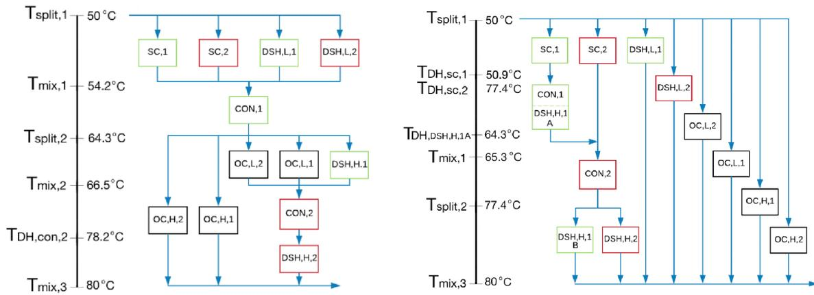
Figure 5: Two possible heat exchanger configurations reaching high COP.
