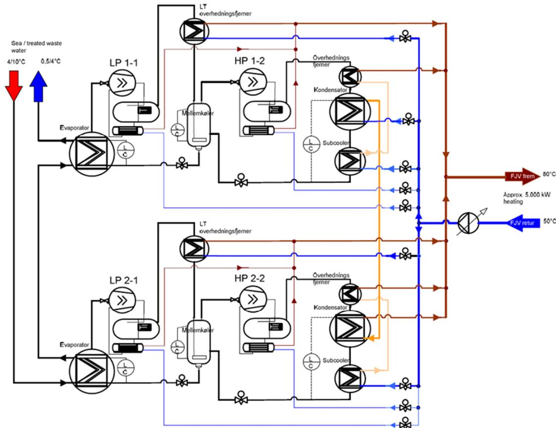
Figure 3: SVAF 2-stage heat pump design
