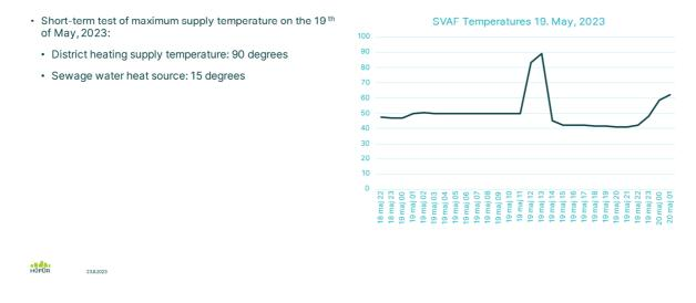
Figure 6: Performance test – Sewage water 2023: Maximum supply temperature
