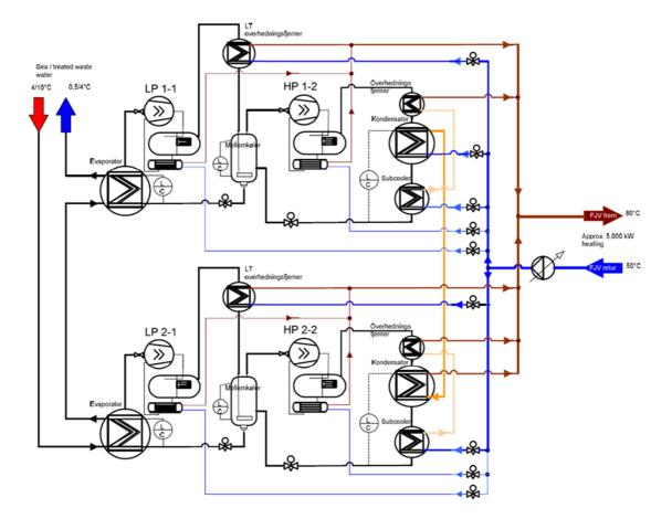
Figure 3: SVAF 2-stage heat pump design
