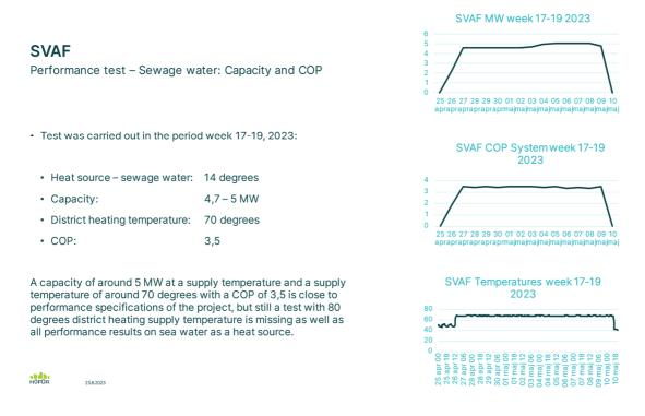
Figure 5: Performance test – Sewage water 2023: Capacity and COP
